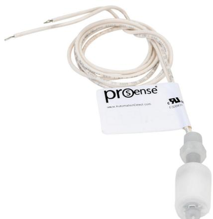
ProSense float liquid level switch, vertical top mount, 1.88in insertion length, 0.75in diameter float, polypropylene wetted parts, -40 to 221 deg F, 1/8in male NPT process connection, SPST reed switch, N.C.
