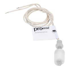
ProSense float liquid level switch, vertical top mount, 1.88in insertion length, 0.75in diameter float, polypropylene wetted parts, -40 to 221 deg F, 1/8in male NPT process connection, SPST reed switch, N.C.
