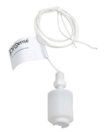
ProSense float liquid level switch, vertical top mount, 1.87in insertion length, 1.12in diameter float, Teflon wetted parts, -40 to 302 deg F, 1/8in male NPT process connection, SPST reed switch, N.C.
