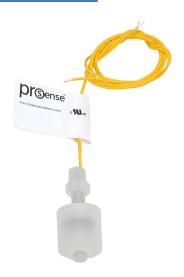
ProSense float liquid level switch, vertical top mount, 1.63in insertion length, 1.0in diameter float, Kynar wetted parts, -40 to 221 deg F, 1/8in male NPT process connection, SPST reed switch, N.O./N.C. selectable.
