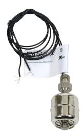
ProSense float liquid level switch, vertical top mount, 1.63in insertion length, 1.13in diameter float, 316 stainless steel wetted parts, -40 to 392 deg F, 1/8in male NPT process connection, SPST reed switch, N.O./N.C. selectable.
