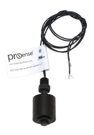
ProSense float liquid level switch, vertical top mount, 1.63in insertion length, 1.0in diameter float, Buna-N, polybutylene wetted parts, -40 to 221 deg F, 1/8in male NPT process connection, SPST reed switch, N.O./N.C. selectable.
