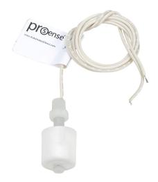
ProSense float liquid level switch, vertical top mount, 1.63in insertion length, 1.0in diameter float, polypropylene wetted parts, -40 to 221 deg F, 1/8in male NPT process connection, SPST reed switch, N.O./N.C. selectable.
