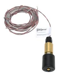
ProSense float liquid level switch, suspendible/submersible mount, 1.44in diameter slosh shield float, Buna-N, brass, polybutylene, halar wetted parts, -40 to 221 deg F, SPST reed switch, N.O./N.C. selectable.
