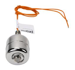
ProSense float liquid level switch, vertical top mount, 2.63in insertion length, 2.13in diameter float, 316 stainless steel wetted parts, -40 to 482 deg F, 1/4in male NPT process connection, SPST reed switch, N.O./N.C. selectable.
