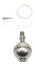
ProSense float liquid level switch, vertical top mount, 2.63in insertion length, 2.05in diameter float, 316 stainless steel wetted parts, -40 to 392 deg F, 1/4in male NPT process connection, SPST reed switch, N.O./N.C. selectable.
