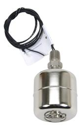
ProSense float liquid level switch, vertical top mount, 2.63in insertion length, 2.13in diameter float, 316 stainless steel wetted parts, -40 to 392 deg F, 1/4in male NPT process connection, SPST reed switch, N.O./N.C. selectable.
