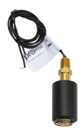
ProSense float liquid level switch, vertical top mount, 2.63in insertion length, 1.25in diameter float, Buna-N, brass wetted parts, -40 to 221 deg F, 1/4in male NPT process connection, SPST reed switch, N.O./N.C. selectable.
