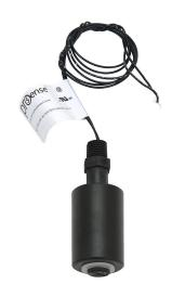
ProSense float liquid level switch, vertical top mount, 2.63in insertion length, 1.25in diameter float, Buna-N, polybutylene wetted parts, -40 to 221 deg F, 1/4in male NPT process connection, SPST reed switch, N.O./N.C. selectable.
