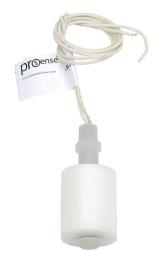
ProSense float liquid level switch, vertical top mount, 2.63in insertion length, 1.5in diameter float, polypropylene wetted parts, -40 to 221 deg F, 1/4in male NPT process connection, SPST reed switch, N.O./N.C. selectable.
