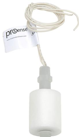
ProSense float liquid level switch, vertical top mount, 2.63in insertion length, 1.5in diameter float, polypropylene wetted parts, -40 to 221 deg F, 1/4in male NPT process connection, SPST reed switch, N.O./N.C. selectable.
