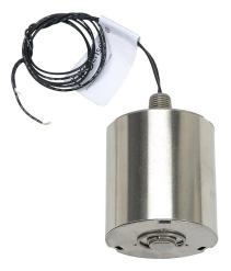
ProSense float liquid level switch, vertical top mount, 2.63in insertion length, 2.38in diameter slosh shield float, 316 stainless steel wetted parts, -40 to 392 deg F, 1/4in male NPT process connection, SPST reed switch, N.O./N.C. selectable.
