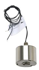
ProSense float liquid level switch, vertical top mount, 1.63in insertion length, 1.90in diameter slosh shield float, 316 stainless steel wetted parts, -40 to 392 deg F, 1/8in male NPT process connection, SPST reed switch, N.O./N.C. selectable.
