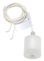
ProSense float liquid level switch, vertical top mount, 1.69in insertion length, 1.44in diameter slosh shield float, polypropylene wetted parts, -40 to 221 deg F, 1/8in male NPT process connection, SPST reed switch, N.O./N.C. selectable.
