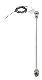
ProSense float liquid level switch, vertical top mount, 32in insertion length, 0.9in diameter float, 316 stainless steel wetted parts, -40 to 302 deg F, 3/4in male NPT pipe plug process connection, (1) SPST reed switch, N.O. and (1) SPST reed switch, N.C.
