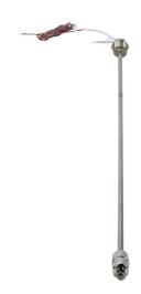
ProSense float liquid level switch, vertical top mount, 32in insertion length, 0.9in diameter float, 316 stainless steel wetted parts, -40 to 302 deg F, 3/4in male NPT pipe plug process connection, SPST reed switch, N.C.
