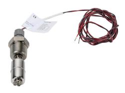
ProSense float liquid level switch, vertical top mount, 2in insertion length, 0.9in diameter float, 316 stainless steel wetted parts, -40 to 302 deg F, 3/4in male NPT pipe plug process connection, SPST reed switch, N.O.
