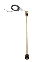
ProSense float liquid level switch, vertical top mount, 32in insertion length, 0.9in diameter float, Buna-N, brass wetted parts, -40 to 221 deg F, 3/4in male NPT pipe plug process connection, (1) SPST reed switch, N.O. and (1) SPST reed switch, N.C.
