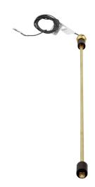
ProSense float liquid level switch, vertical top mount, 32in insertion length, 0.9in diameter float, Buna-N, brass wetted parts, -40 to 221 deg F, 3/4in male NPT pipe plug process connection, (1) SPST reed switch, N.O. and (1) SPST reed switch, N.C.
