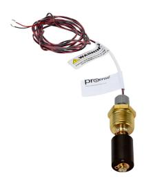
ProSense float liquid level switch, vertical top mount, 2in insertion length, 0.9in diameter float, Buna-N, brass wetted parts, -40 to 221 deg F, 3/4in male NPT pipe plug process connection, SPST reed switch, N.O.
