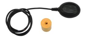
ProSense float liquid level tilt switch, suspendible/submersible mount, EPDM rubber oval float, EPDM rubber oval, polypropylene, PVC wetted parts, 32 to 158 deg F, mercury-free SPDT switch.
