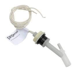
ProSense float liquid level switch, horizontal side mount, 3.31in insertion length, 0.65in diameter float, polypropylene, nitrile wetted parts, -40 to 221 deg F, 5/8-11 male UNC with gasket, washer and nut process connection, SPST reed switch, N.O./N.C. selectable.
