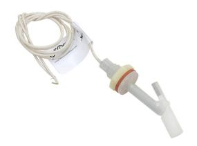
ProSense float liquid level switch, horizontal side mount, 2.84in insertion length, 0.65in diameter float, polypropylene, silicone wetted parts, -40 to 221 deg F, 5/8-11 male UNC with washer and nut process connection, SPST reed switch, N.O./N.C. selectable.
