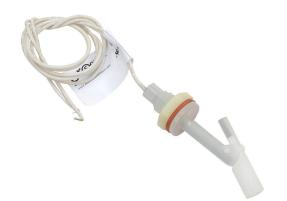
ProSense float liquid level switch, horizontal side mount, 2.84in insertion length, 0.65in diameter float, polypropylene, silicone wetted parts, -40 to 221 deg F, 5/8-11 male UNC with washer and nut process connection, SPST reed switch, N.O./N.C. selectable.
