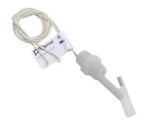
ProSense float liquid level switch, horizontal side mount, 2.75in insertion length, 0.65in diameter float, polypropylene wetted parts, -40 to 221 deg F, dual 1/2in male NPT process connection, SPST reed switch, N.O./N.C. selectable.
