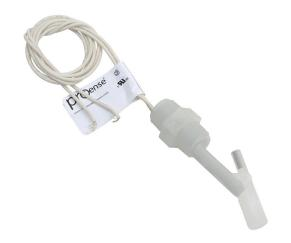
ProSense float liquid level switch, horizontal side mount, 2.75in insertion length, 0.65in diameter float, polypropylene wetted parts, -40 to 221 deg F, dual 1/2in male NPT process connection, SPST reed switch, N.O./N.C. selectable.
