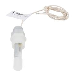
ProSense float liquid level switch, horizontal side mount, 2.75in insertion length, 0.65in diameter float, polypropylene wetted parts, -40 to 221 deg F, 3/4in male NPT process connection, SPST reed switch, N.O./N.C. selectable.
