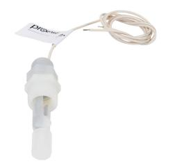
ProSense float liquid level switch, horizontal side mount, 2.75in insertion length, 0.65in diameter float, polypropylene wetted parts, -40 to 221 deg F, 3/4in male NPT process connection, SPST reed switch, N.O./N.C. selectable.
