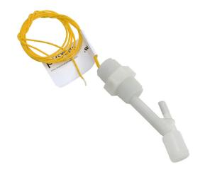
ProSense float liquid level switch, horizontal side mount, 2.75in insertion length, 0.65in diameter float, Kynar wetted parts, -40 to 221 deg F, dual 1/2in male NPT process connection, SPST reed switch, N.O./N.C. selectable.
