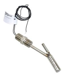
ProSense float liquid level switch, horizontal side mount, 4.6in insertion length, 0.63in diameter float, 316 stainless steel wetted parts, -40 to 392 deg F, dual 1/2in male NPT process connection, SPST reed switch, N.O./N.C. selectable.
