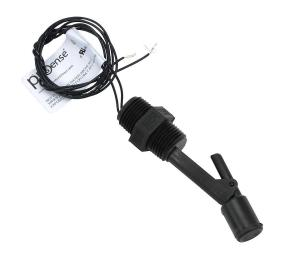
ProSense float liquid level switch, horizontal side mount, 2.75in insertion length, 0.65in diameter float, polybutylene wetted parts, -40 to 266 deg F, dual 1/2in male NPT process connection, SPST reed switch, N.O./N.C. selectable.
