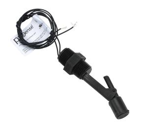
ProSense float liquid level switch, horizontal side mount, 2.75in insertion length, 0.65in diameter float, polybutylene wetted parts, -40 to 266 deg F, dual 1/2in male NPT process connection, SPST reed switch, N.O./N.C. selectable.
