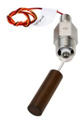
ProSense float liquid level switch, horizontal side mount, 4.43in insertion length, 0.92in diameter float, Buna-N, 304 stainless steel, Teflon, Ceramic wetted parts, -40 to 221 deg F, 1in male NPT process connection, SPDT reed switch, N.O./N.C. selectable.
