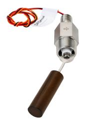
ProSense float liquid level switch, horizontal side mount, 4.43in insertion length, 0.92in diameter float, Buna-N, 304 stainless steel, Teflon, Ceramic wetted parts, -40 to 221 deg F, 1in male NPT process connection, SPDT reed switch, N.O./N.C. selectable.
