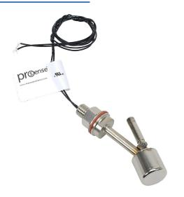
ProSense float liquid level switch, horizontal side mount, 3.19in insertion length, 1.0in diameter float, 316 stainless steel wetted parts, -40 to 392 deg F, 1/2-13 male UNC with washers and nut process connection, SPST reed switch, N.O./N.C. selectable.
