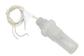
ProSense float liquid level switch, horizontal side mount, 2.84in insertion length, 1.12in diameter slosh shield float, polypropylene wetted parts, -40 to 221 deg F, 1in male NPT x 1/2in male NPT process connection, SPST reed switch, N.O./N.C. selectable.
