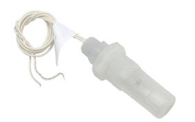
ProSense float liquid level switch, horizontal side mount, 2.84in insertion length, 1.12in diameter slosh shield float, polypropylene wetted parts, -40 to 221 deg F, 1in male NPT x 1/2in male NPT process connection, SPST reed switch, N.O./N.C. selectable.
