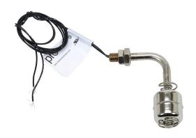
ProSense float liquid level switch, horizontal side mount, 2.18in insertion length, 1.13in diameter float, 316 stainless steel wetted parts, -40 to 392 deg F, 3/8-24 male UNC with nut process connection, SPST reed switch, N.O./N.C. selectable.
