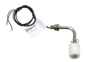
ProSense float liquid level switch, horizontal side mount, 2.11in insertion length, 1.0in diameter float, polypropylene, 316 stainless steel wetted parts, -40 to 221 deg F, 3/8-24 male UNC with nut process connection, SPST reed switch, N.O./N.C. selectable.
