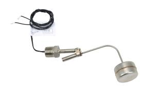
ProSense float liquid level switch, horizontal side mount, 5.77in insertion length, 1.60in diameter float, 316 stainless steel wetted parts, -40 to 392 deg F, 1/2in male NPT process connection, SPST reed switch, N.O./N.C. selectable.
