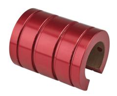
PBC Simplicity series open plain bearing, PTFE, 1-1/4in inside diameter, 2in outside diameter, 2-5/8in overall length, 0.0005in running clearance. For use with 1-1/4in diameter PBC shafts.
