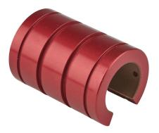
PBC Simplicity series open plain bearing, PTFE, 1in inside diameter, 1-9/16in outside diameter, 2-1/4in overall length, 0.0005in running clearance. For use with 1in diameter PBC shafts.
