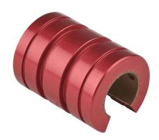
PBC Simplicity series open plain bearing, PTFE, 5/8in inside diameter, 1-1/8in outside diameter, 1-1/2in overall length, 0.0005in running clearance. For use with 5/8in diameter PBC shafts.
