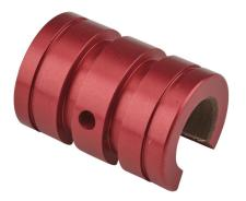
PBC Simplicity series open plain bearing, PTFE, 1/2in inside diameter, 7/8in outside diameter, 1-1/4in overall length, 0.0005in running clearance. For use with 1/2in diameter PBC shafts.
