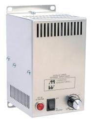
Hammond enclosure heater, axial fan, 670/800W heating capacity, incoloy tubular heating element, 220-240 VAC operating voltage, 50/60 Hz, adjustable thermostat, N.C. (open on rise) 0 to 100 deg F, panel mount.
