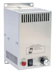
Hammond enclosure heater, axial fan, 800W heating capacity, incoloy tubular heating element, 120 VAC operating voltage, 60 Hz, adjustable thermostat, N.C. (open on rise) 0 to 100 deg F, panel mount.
