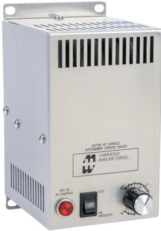
Hammond enclosure heater, axial fan, 335/400W heating capacity, incoloy tubular heating element, 220-240 VAC operating voltage, 50/60 Hz, adjustable thermostat, N.C. (open on rise) 0 to 100 deg F, panel mount.
