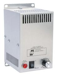
Hammond enclosure heater, axial fan, 400W heating capacity, incoloy tubular heating element, 120 VAC operating voltage, 60 Hz, adjustable thermostat, N.C. (open on rise) 0 to 100 deg F, panel mount.
