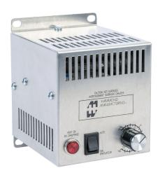
Hammond enclosure heater, axial fan, 165/200W heating capacity, incoloy tubular heating element, 220-240 VAC operating voltage, 50/60 Hz, adjustable thermostat, N.C. (open on rise) 0 to 100 deg F, panel mount.
