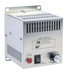
Hammond enclosure heater, axial fan, 200W heating capacity, incoloy tubular heating element, 120 VAC operating voltage, 60 Hz, adjustable thermostat, N.C. (open on rise) 0 to 100 deg F, panel mount.
