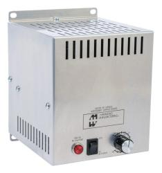
Hammond enclosure heater, axial fan, 1300W heating capacity, incoloy tubular heating element, 120 VAC operating voltage, 60 Hz, adjustable thermostat, N.C. (open on rise) 0 to 100 deg F, panel mount.
