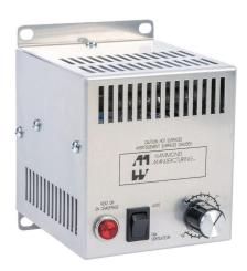
Hammond enclosure heater, axial fan, 105/125W heating capacity, incoloy tubular heating element, 220-240 VAC operating voltage, 50/60 Hz, adjustable thermostat, N.C. (open on rise) 0 to 100 deg F, panel mount.
