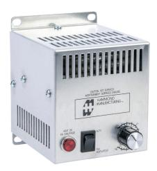
Hammond enclosure heater, axial fan, 125W heating capacity, incoloy tubular heating element, 120 VAC operating voltage, 60 Hz, adjustable thermostat, N.C. (open on rise) 0 to 100 deg F, panel mount.
