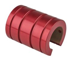
PBC Simplicity series open plain bearing, PTFE, 1-1/4in inside diameter, 2in outside diameter, 2-5/8in overall length, 0.0015in running clearance. For use with 1-1/4in diameter PBC shafts.
