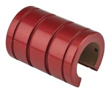
PBC Simplicity series open plain bearing, PTFE, 1in inside diameter, 1-9/16in outside diameter, 2-1/4in overall length, 0.0015in running clearance. For use with 1in diameter PBC shafts.
